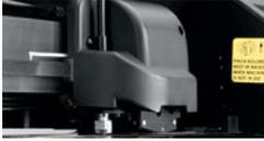
Fig. 3.11-4: Cutting head with sensor and tangential knife
