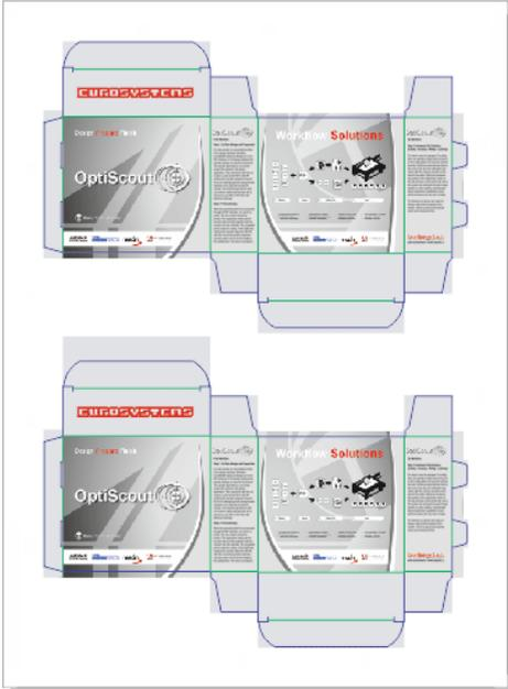
Fig. 10.1-6: Cut crease contour located above print data
